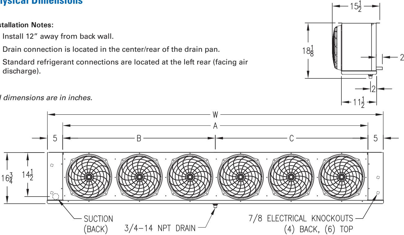
**NOTE:** Refrigerant and electrical connection locations have been changed for the Next-Gen All-Temp design. Standard connections are now opposite of the legacy All-Temp models.
