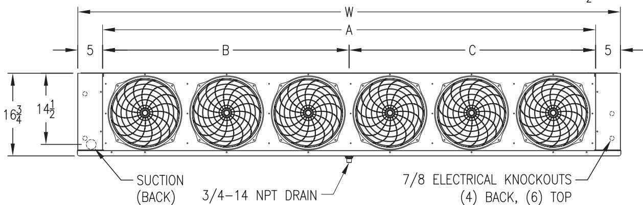
**NOTE:** Refrigerant and electrical connection locations have been changed for the Next-Gen All-Temp design. Standard connections are now opposite of the legacy Super-Flo models.
